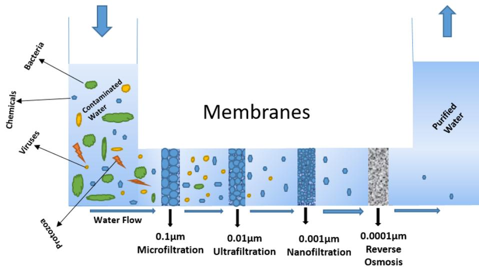
**Fig 9: Membrane filters and representative water contaminants removed**
