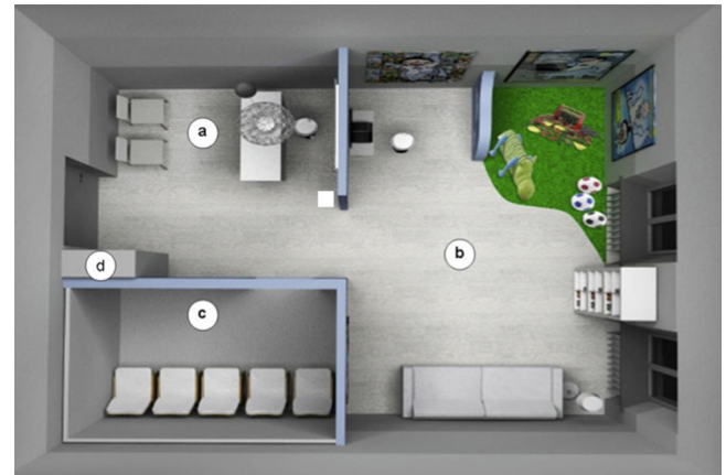
Fig. 1. “Salt Clinic”. 3D design: reception/welcome area (a); waiting room with children's recreation area (b); “Aerosal ® ” halotherapy room (c). ENT Care Unit (d). Cabinet containing the Dry Salt Aerosol Generator – University General Hospital – Bari (Italy).
